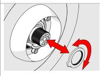
4. Remove the lower brass ring (temperature setting ring) and rotate the brass ring clockwise to increase temperature or anti-clockwise to decrease. Refit to spline in new position.
