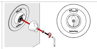
Fit the handle and fasten so the arrow shape on top of the handle matches the marking on the faceplate.
