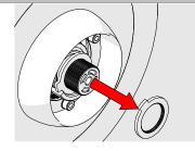
Remove the upper brass ring. Make sure the control rod doesn't rotate during the next steps.
