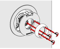
7. Fit the inner faceplate into the outer faceplate. Ensure the marking on the top of the plate is positioned correctly.
