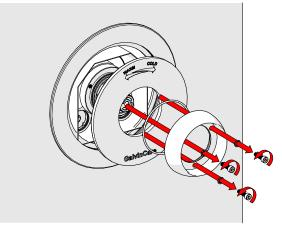
To isolate the shower, remove the handle and flange by unscrewing and carefully remove the inner faceplate and flange o-ring. (As shown)
