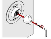
Unscrew the tamper proof screw from handle. Pull out handle assembly from the body
